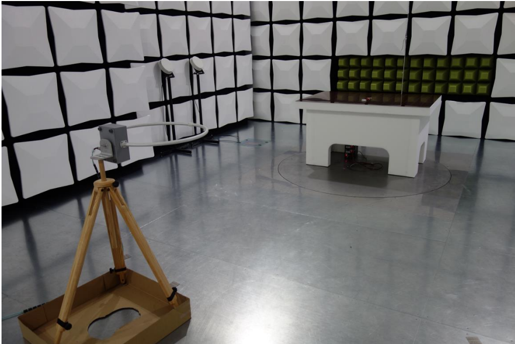
Photo of test setup for 9kHz – 30MHz Ground-parallel position
