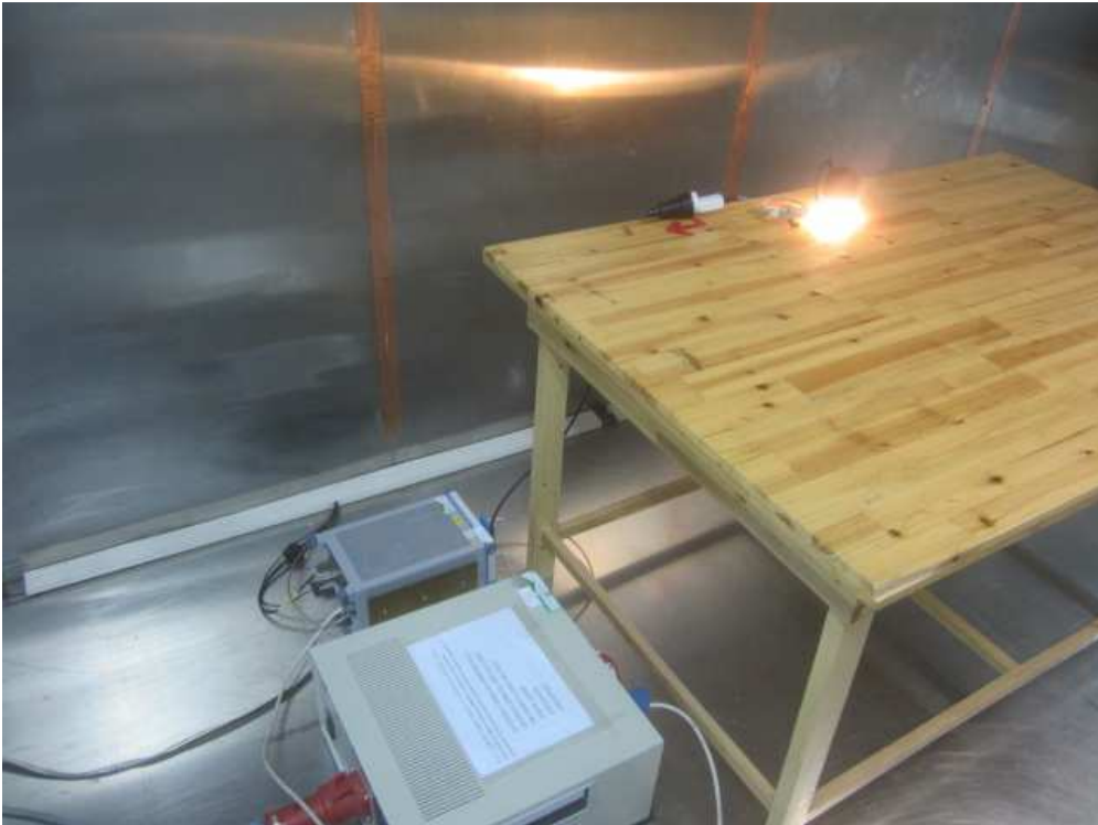
Photograph 2: Set-up for measurement of radiated emission
