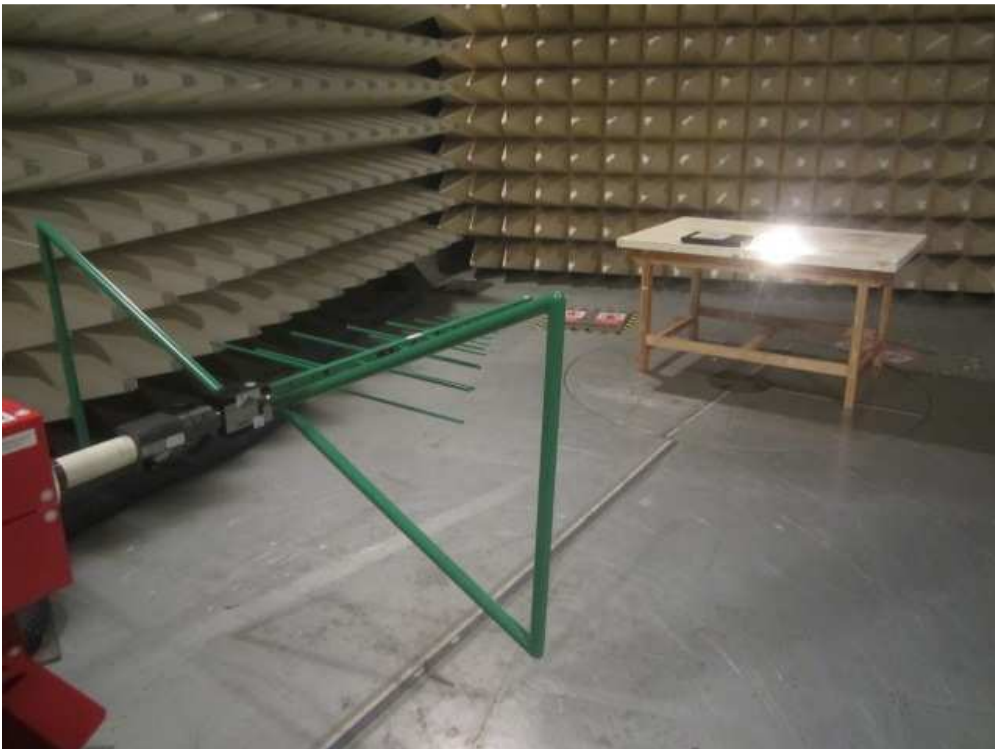
Photograph 2: Set-up for measurement of radiated emission
