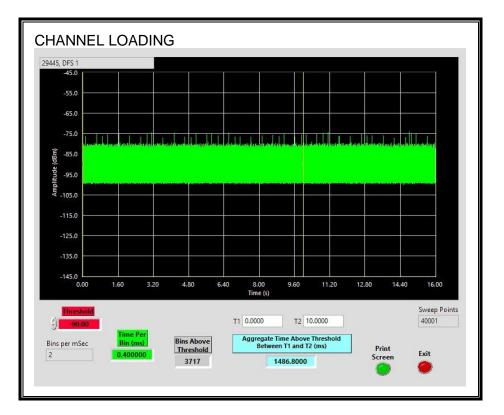
The level of traffic loading on the channel by the EUT is 14.86% The channel loading is the highest level that the EUT is capable of producing.
