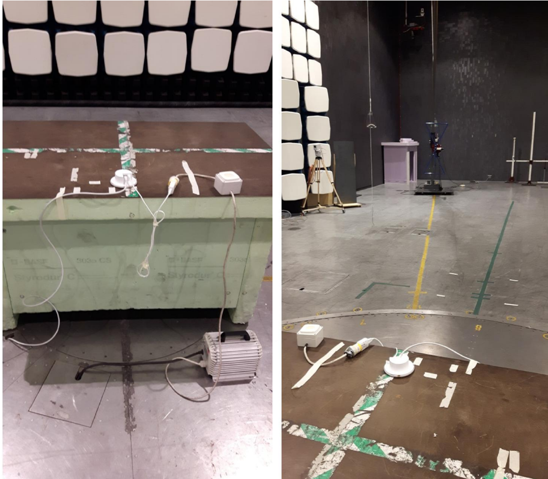
Test set up radiated emission 30 MHz – 1GHz
