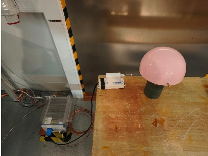
Photograph 1: Set-up for measurement of conducted emission
