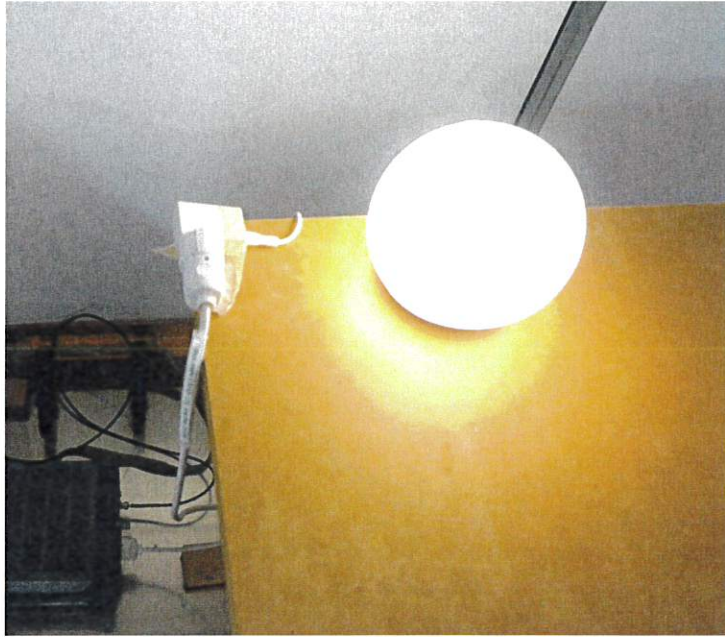
Test setup for conducted emission 150 kHz – 30 MHz
