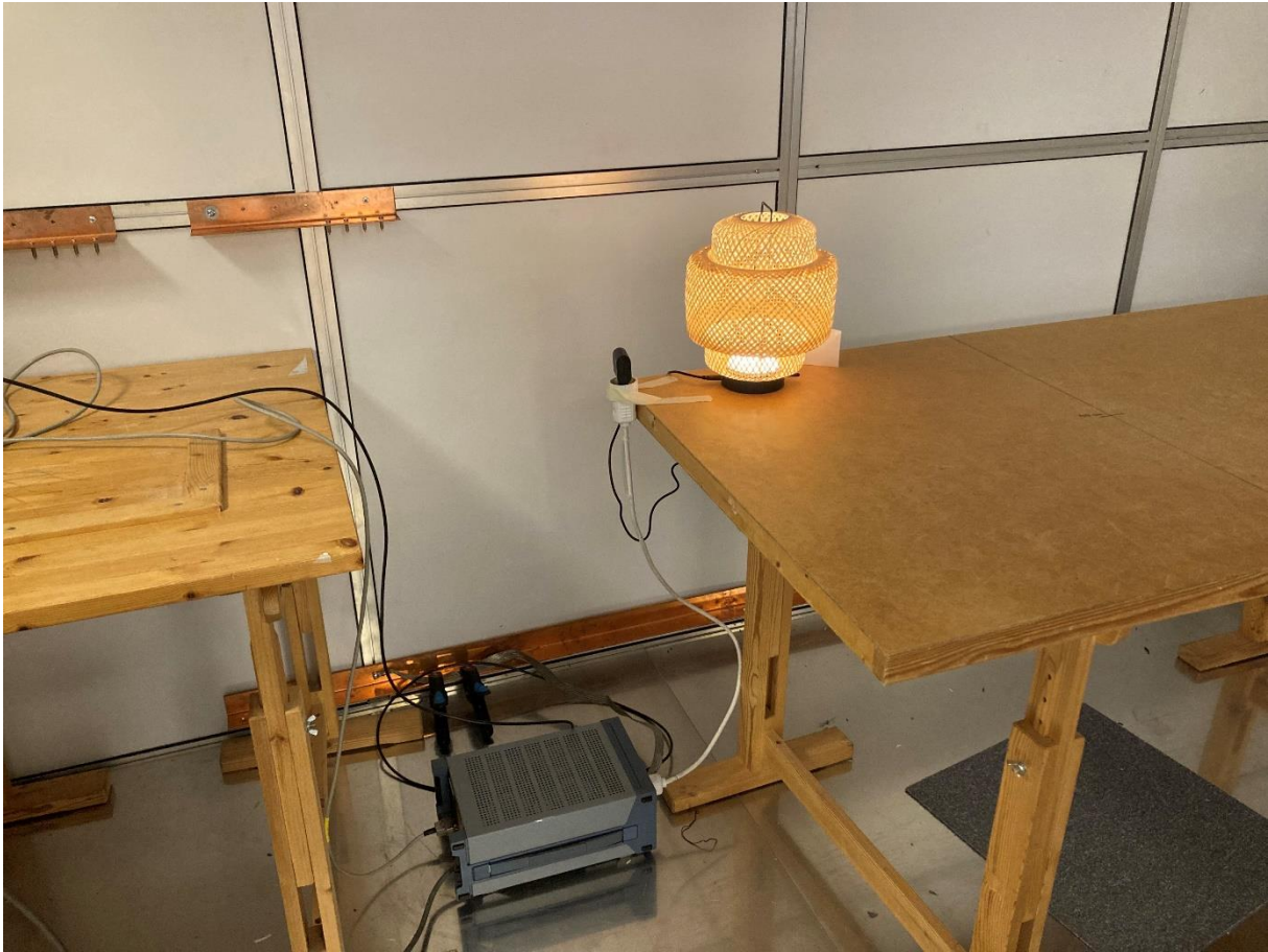
Test setup for conducted emission 150 kHz – 30 MHz
