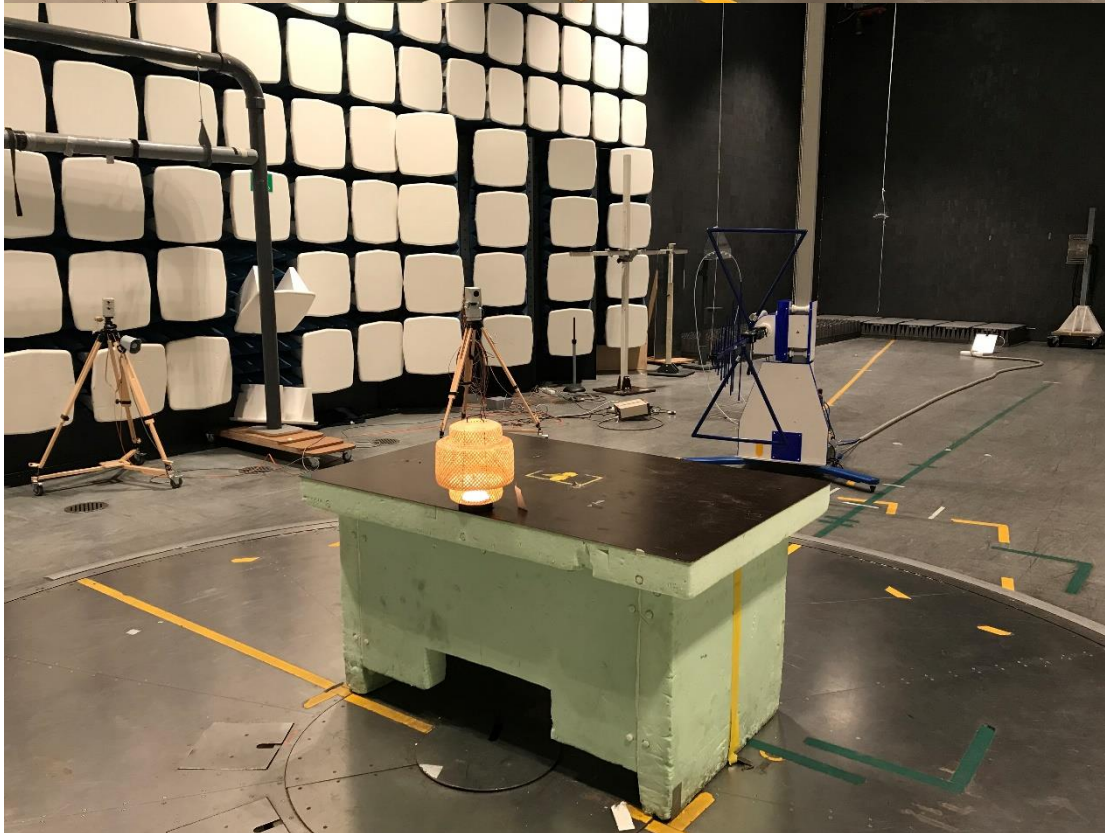
Test set up radiated emission 30 MHz – 1 GHz
