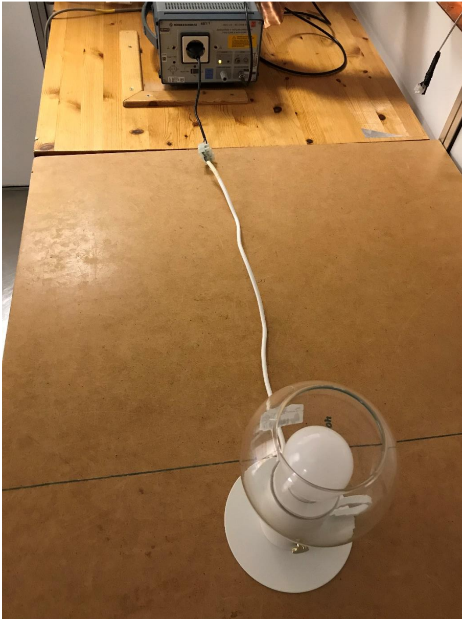
Test setup for conducted emission 150 kHz – 30 MHz
