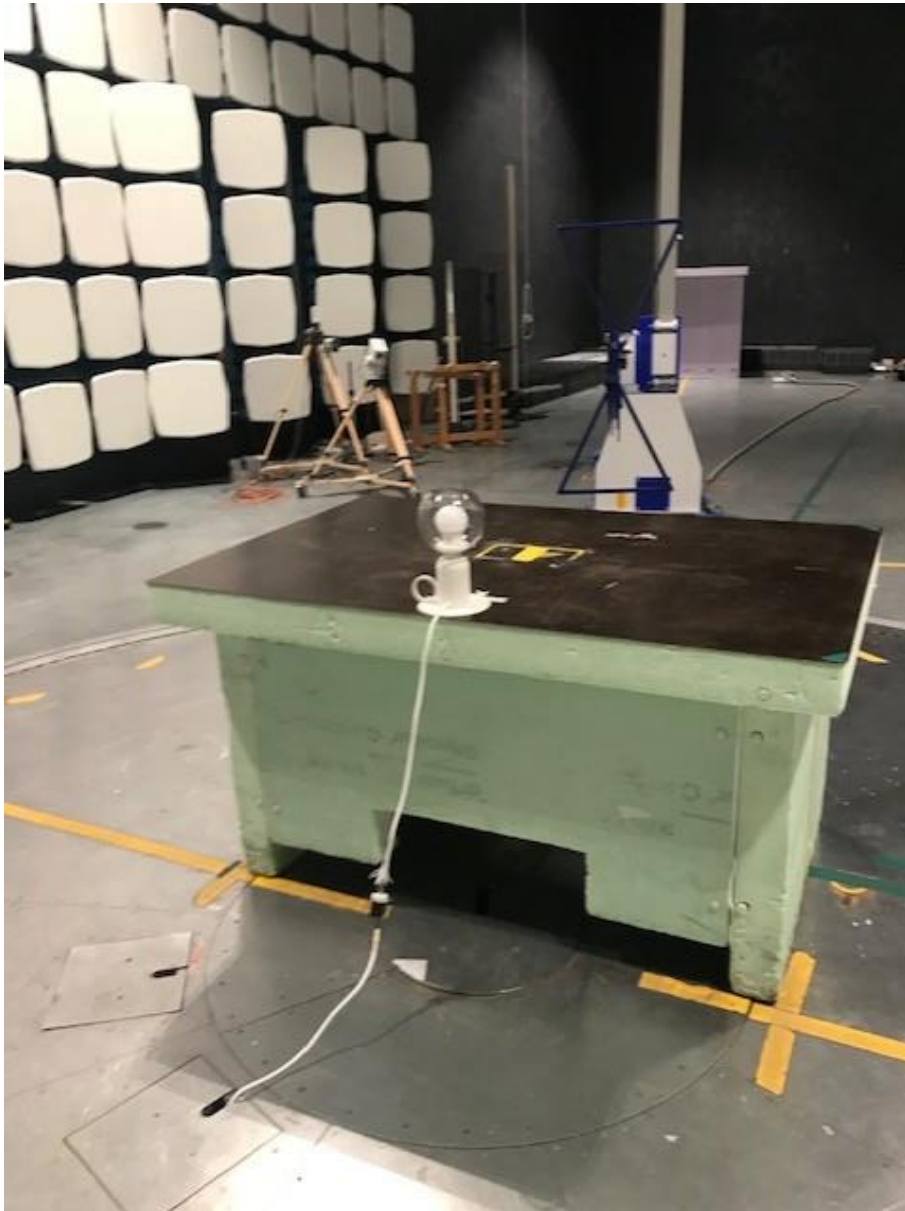
Test set up radiated emission 30 MHz – 1 GHz
