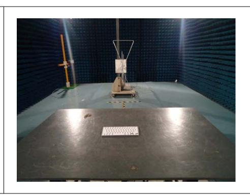
Radiation Emission Test Setup
