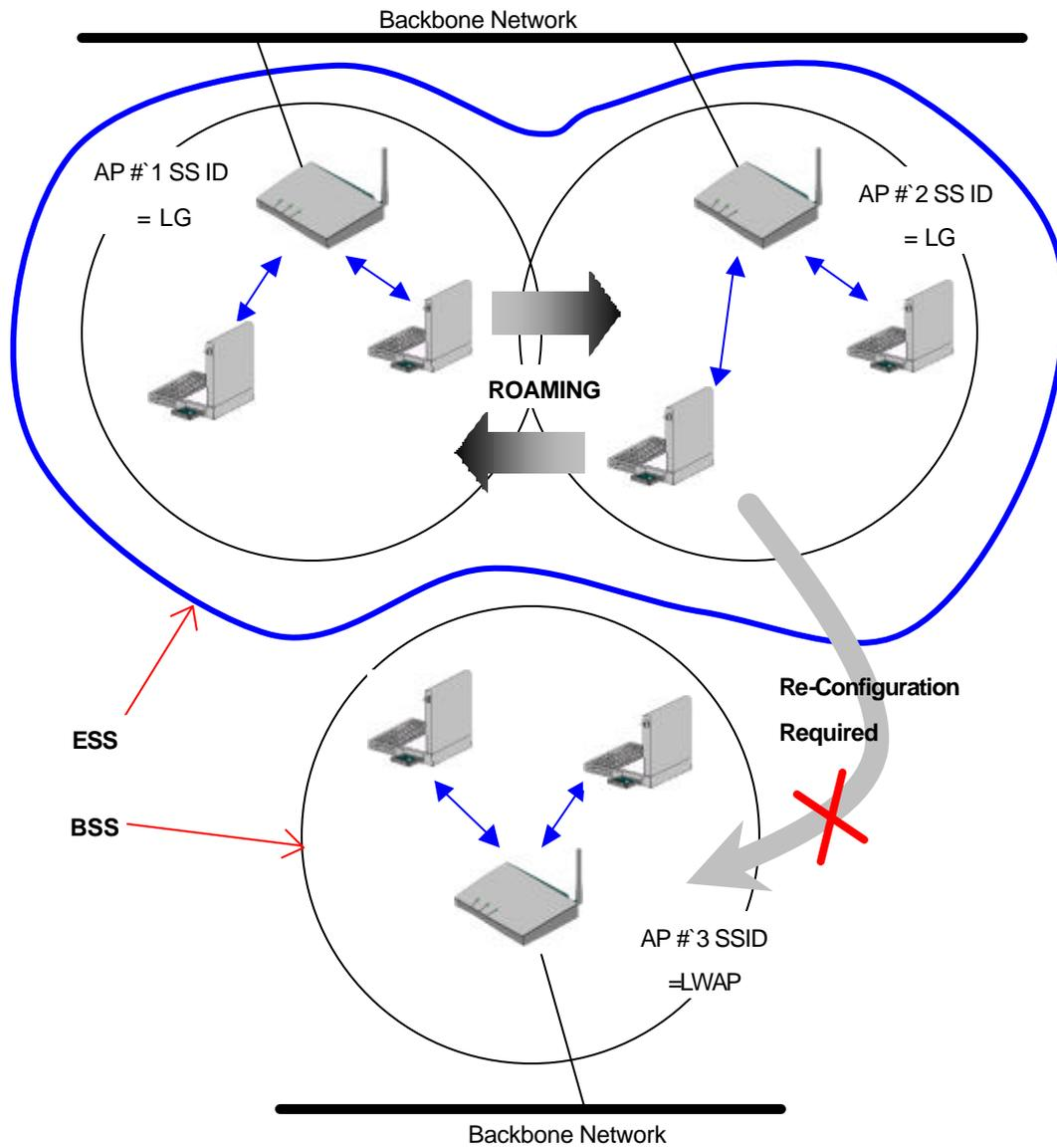
Figure 4. SSID and Roaming
