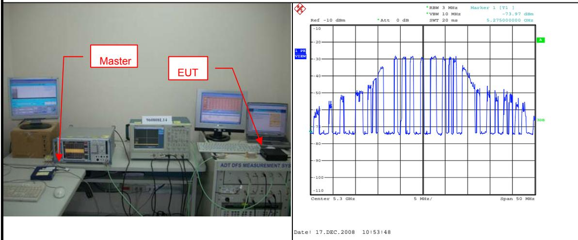
**EUT (Client) links with master on 5500MHz**
