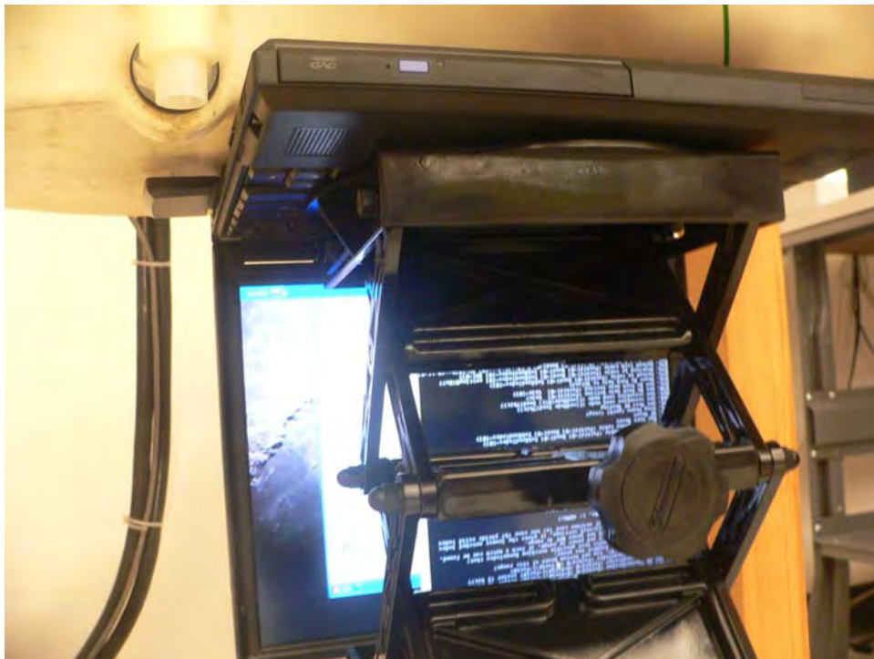
EUT with IBM laptop back touching to the flat phantom Front View
