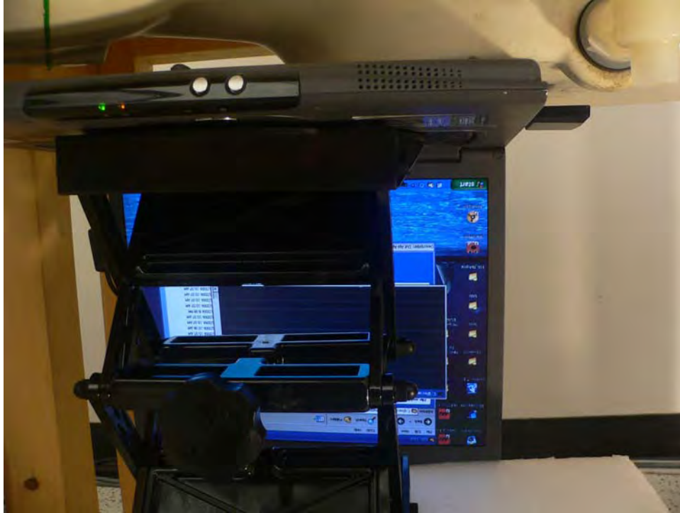
EUT with Acer laptop back touching to the flat phantom Front View
