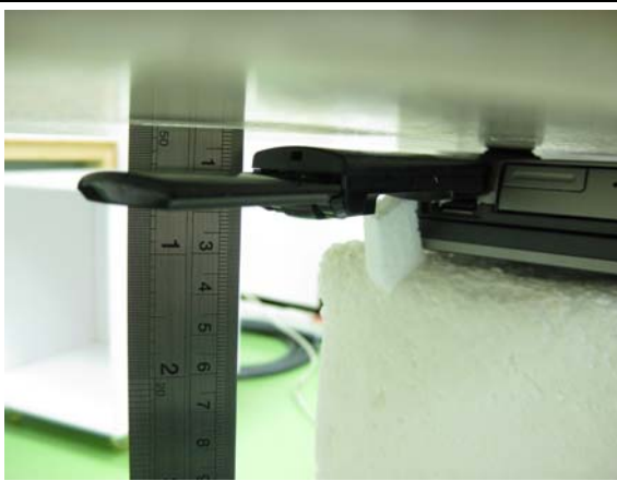
G: The bottom of the EUT face to the phantom with 5mm-separation distance.
