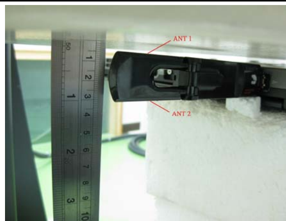
J: The right edge of the EUT face to the phantom with 5mm-separation distance.
