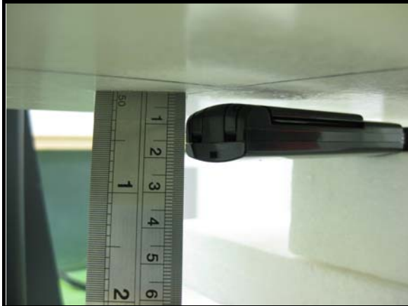
A: The front of the EUT face to the phantom with 5mm-separation distance.
