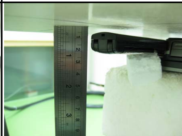
F: The bottom of the EUT face to the phantom with 5mm-separation distance.
