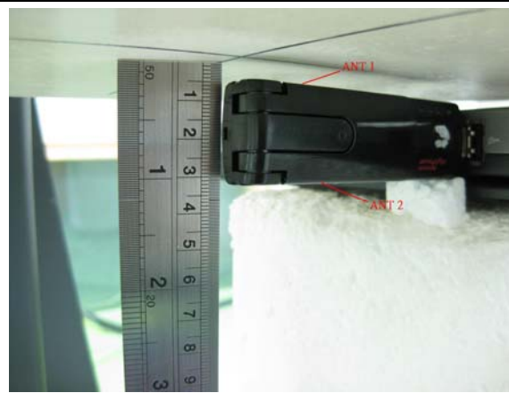
H: The right edge of the EUT face to the phantom with 5mm-separation distance.
