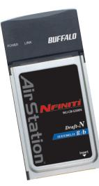
• The WLI-CB-G300N has three internal diversity antennas. External antennas can not be attached to the WLI-CB-G300N.
