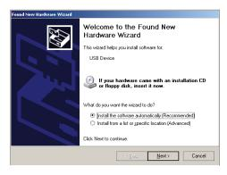
Power on the notebook PC and let it boot into Windows. Plug the Wireless USB Adapter into an available USB port on your PC. The Found New Hardware Wizard will launch automatically.
