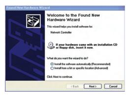
Plug the Wireless USB Adapter or stand into an available USB port on your PC. The Found New Hardware Wizard will launch automatically.
