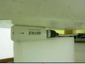
The right of the EUT face to the phantom with 0mmseparation distance (with cable).
