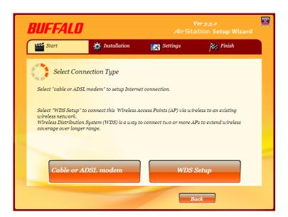
When the below screen appears, select [AOSS configuration] or [Manual Configuration] from [Select WDS Setup method].
