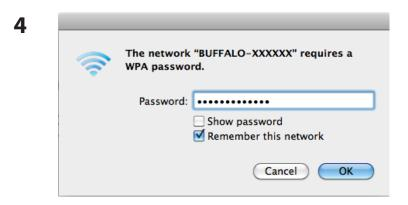
Enter the value for the KEY that was noted in step 1 into the Password entry box, insert a check mark into [Remember this network], and click [OK].
