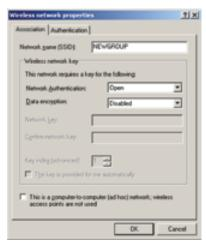
Click the Advanced button to enter an SSID network name or WEP/WPA encryption key, if either is necessary. To add an SSID network name that is not available, click the Add button.
