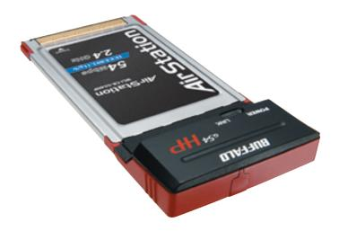
▶ The WLI-CB-G54HP comes with an external antenna connector. Buffalo Technology sells numerous external antennas that are compatible with this card. The connector type is called an MC-Card Connector. Adding an external antenna can further increase the power and range of this device. Please see the Buffalo Technology Web Page (http://www.buffalotech.com) to compare antennas available for your adapter.
