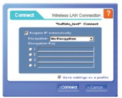
The 'Acquire IP automatically' checkbox tells the client device to obtain an IP automatically from a DHCP server. This is the recommended setting.
