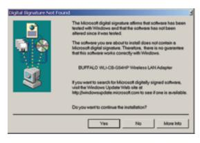
• Windows 2000: If the Digital Signature Not Found page opens, informing that no digital signature exists for the driver you are installing, click the Yes button to continue the installation process. When the Wireless Notebook Adapter is successfully installed, click the Finish button. Restart your computer if prompted.
