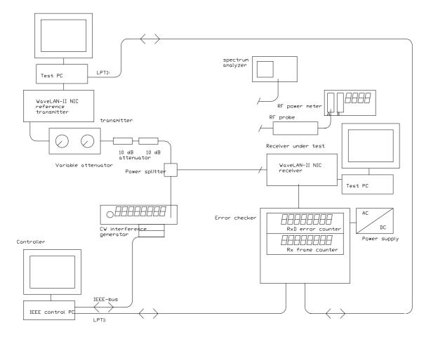
Figure 1, measurement test set-up.
