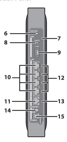
**6 Router button** This button turns the router on and off. The operation mode is changed
