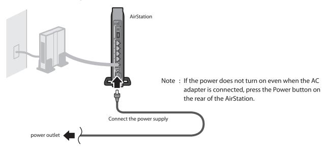
If using a wired LAN, connect the AirStation LAN port and computer using a LAN cable. If using a wireless LAN, connect the computer to the wireless LAN by referring to Chapter 4.
