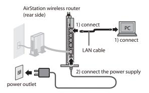
6 Confirm the devices are connected correctly as the below diagram shows.
