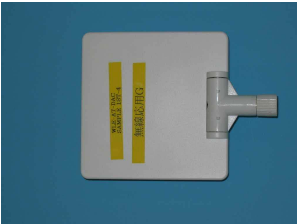
Rear Side of Directional Panel
