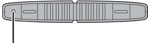
With the AirStation powered on, hold down this button for 3 seconds to return it to factory default settings.
