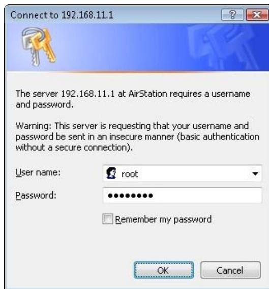
When this screen appears, enter "root" (in lower case) for the user name and the password that you set during initial setup. Click "OK".
