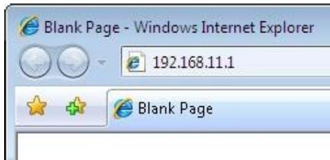
Enter the AirStation's LAN-side IP address in the address field, and press the "Enter" key.
