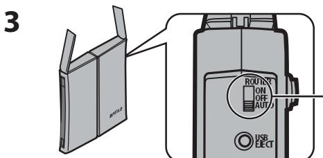
Make sure the mode switch on the back of the AirStation is in the "AUTO" position.
