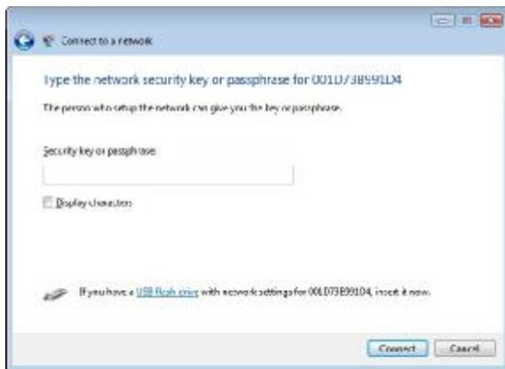
When the screen at left is displayed, enter an encryption key (such as WEP key or pre-shared key) and click "Connect".
