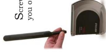
Screw the antenna into the top of your AirStation. It will probably work best if you orient it to point straight up.
