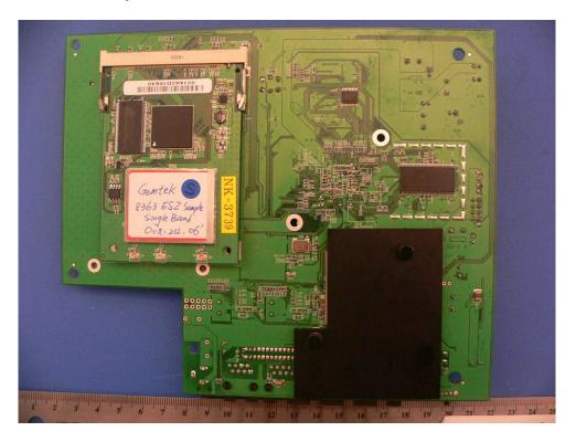
**EUT – RF Board Single Band with RF Shielding (Component Side View)**
