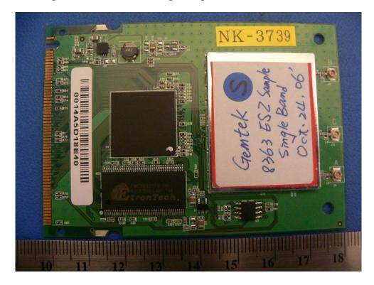
EUT – RF Board Single Band without RF Shielding (Component Side View)
