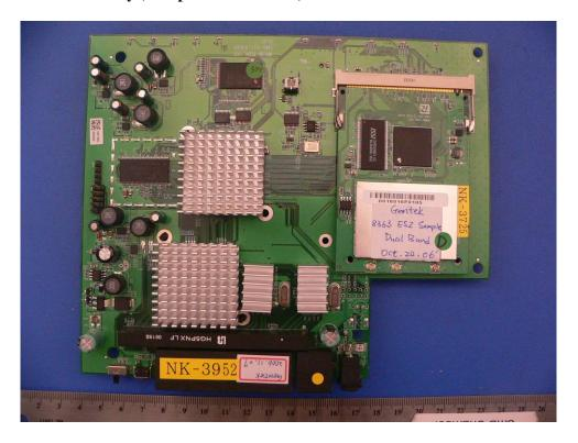
EUT – Main Board Assembly with RF board (Solder Side View)
