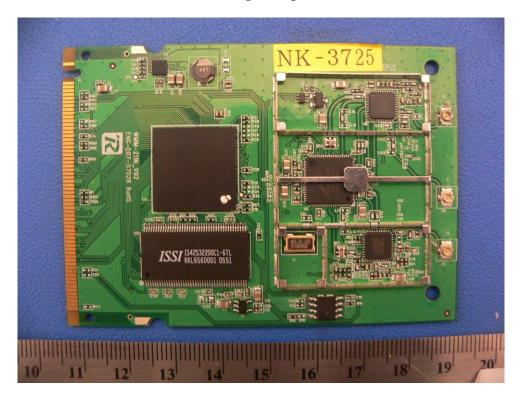
**EUT – RF Board Dual Band (Solder Side View)**
