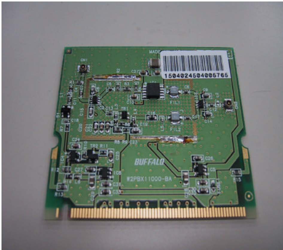
Front View of RF Module Interface Print Circuit Board with Shield Off
