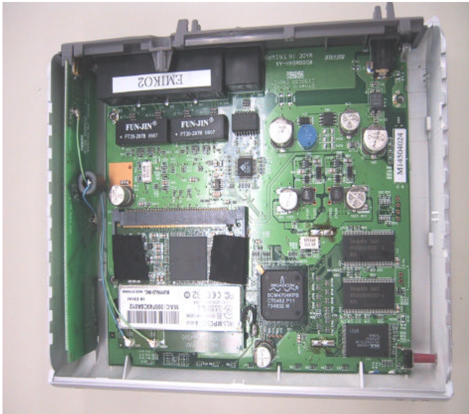
Inside of Enclosure
