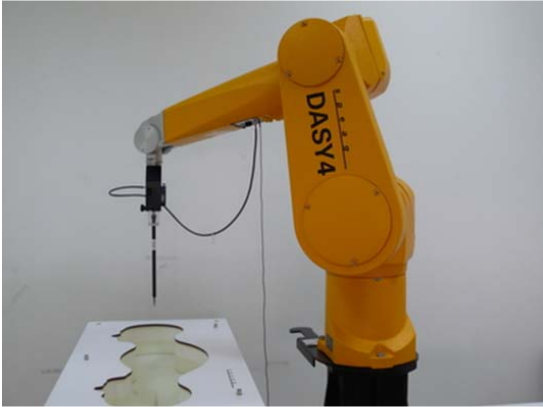
Picture 1: Specific Absorption Rate Test Layout
