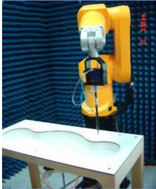
Photo 1: SAR measurement System
