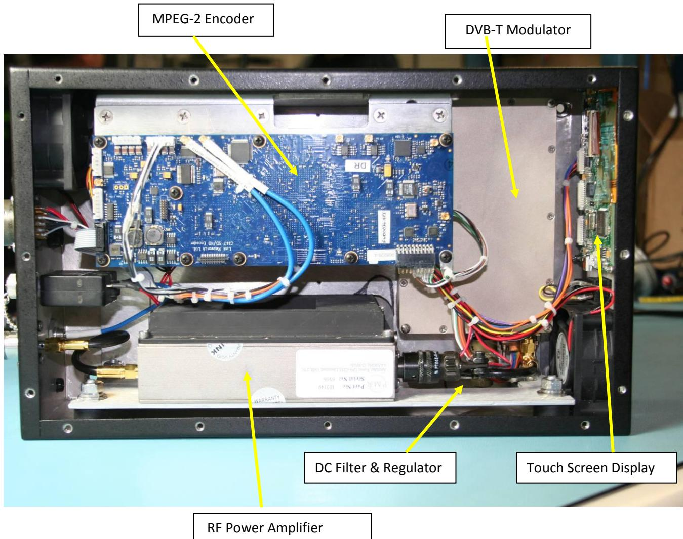
**NOTE: THERE IS ONLY ONE REMOVEABLE COVER. ALL INTERNAL COMPONENTS CAN BE VIEWED AND ACCESSED THROUGH THE SINGLE COVER, AS SHOWN ABOVE.**
