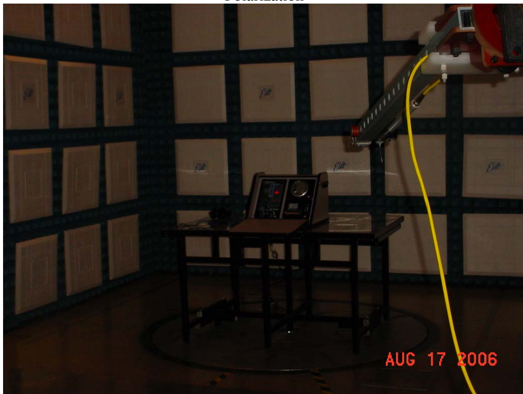
Test Setup for Radiated Emissions, 904MHz to 927MHz – Vertical
