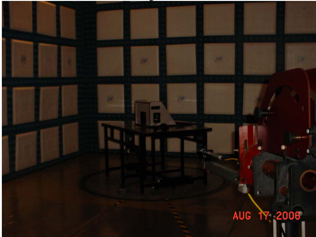
Test Setup for Radiated Emissions, 904MHz to 927MHz– Horizontal Polarization
