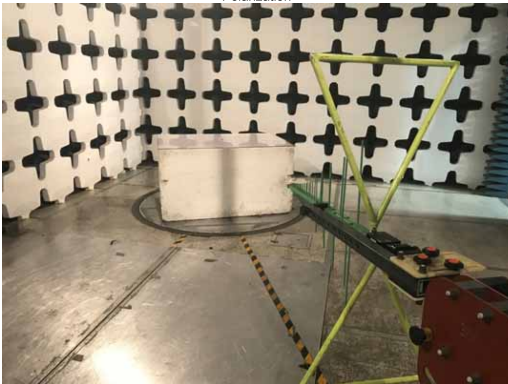
Figure 4 – Test Setup for Radiated Emissions, 30MHz to 1GHz – Vertical Polarization
