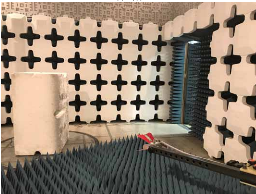
Figure 6 – Test Setup for Radiated Emissions, 1GHz to 25GHz – Vertical Polarization
