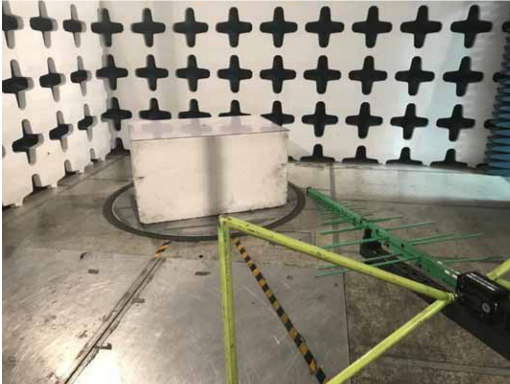
Figure 3 – Test Setup for Radiated Emissions, 30MHz to 1GHz – Horizontal Polarization
