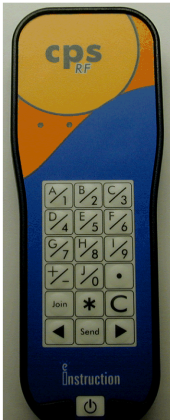
eInstruction cpsRF HE keypad topside. Note uni-body case, single LED indicators and membrane keypad contact type.
