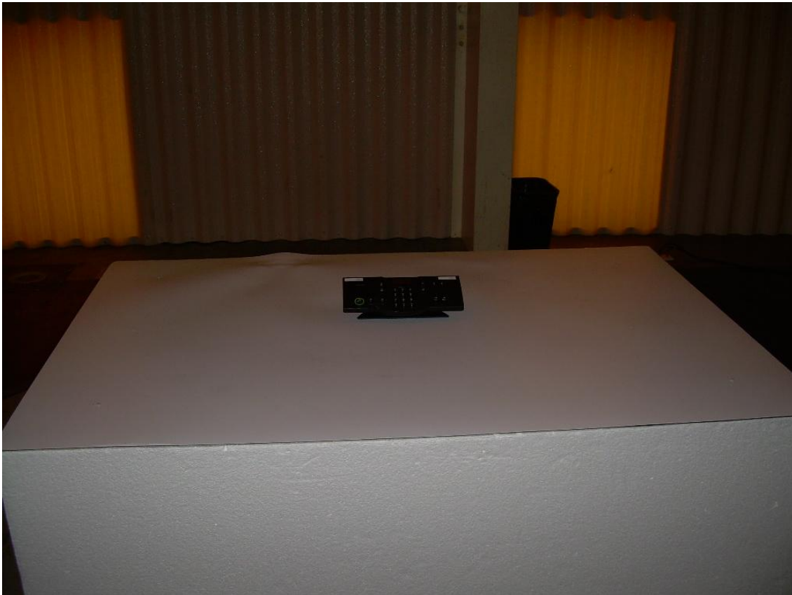
Photograph 1 - Radiated Spurious Emission Worst-Case Setup
