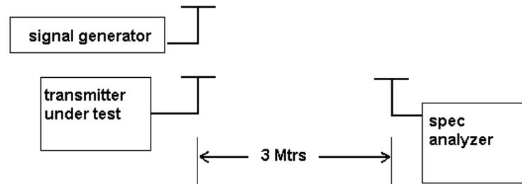
**FIELD STRENGTH OF SPURIOUS EMISSIONS TEST SETUP PHOTO**
