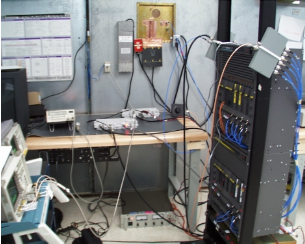
Conducted Spurious Setup at KTL Ottawa Laboratories
