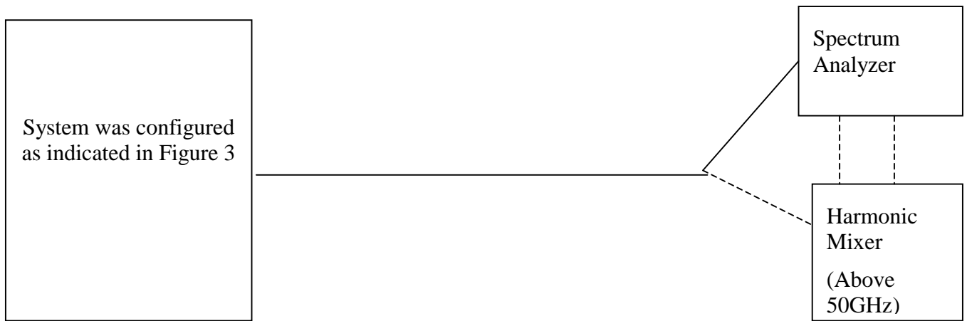
Conducted Spurious measurement setup
