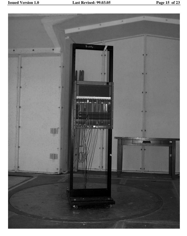
Figure 4-1 Radiated Emissions (Electric Field)
