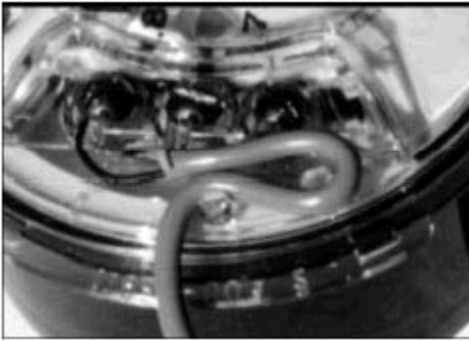
Figure 2.5 Cable Threaded Around Strain Relief Posts
