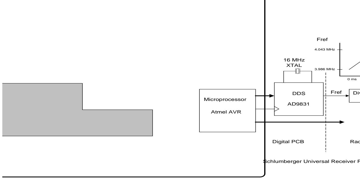
As the drawing above indicates, to incorporate the “fast scan” capability, the receiver uses a DDS synthesizer IC to “drive” our conventional phase locked loop.
