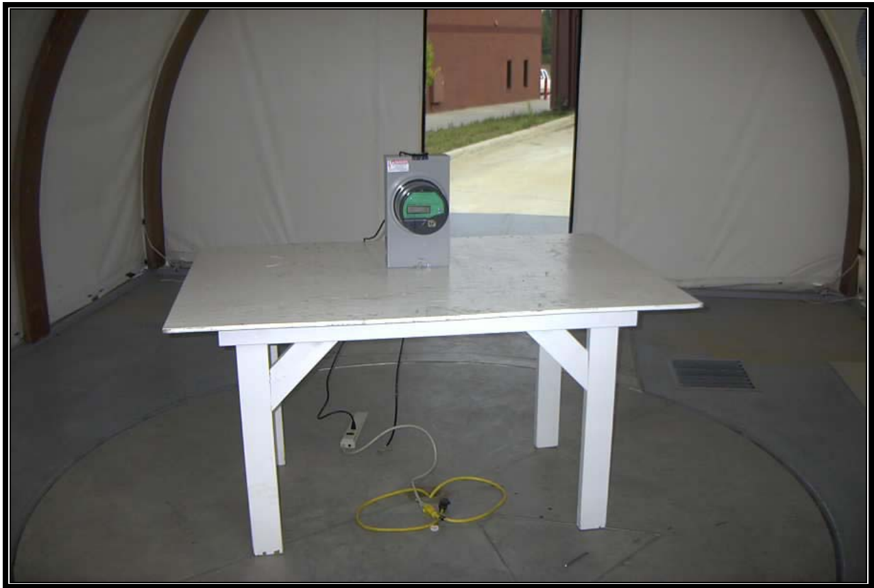
Figure 7.3-1: Radiated Emission Test Setup
