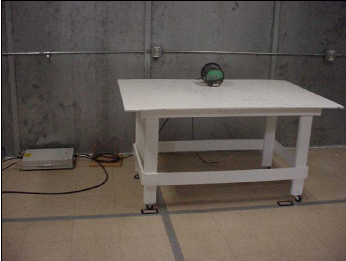
Figure 7.2-2: Conducted Emissions Test Setup
