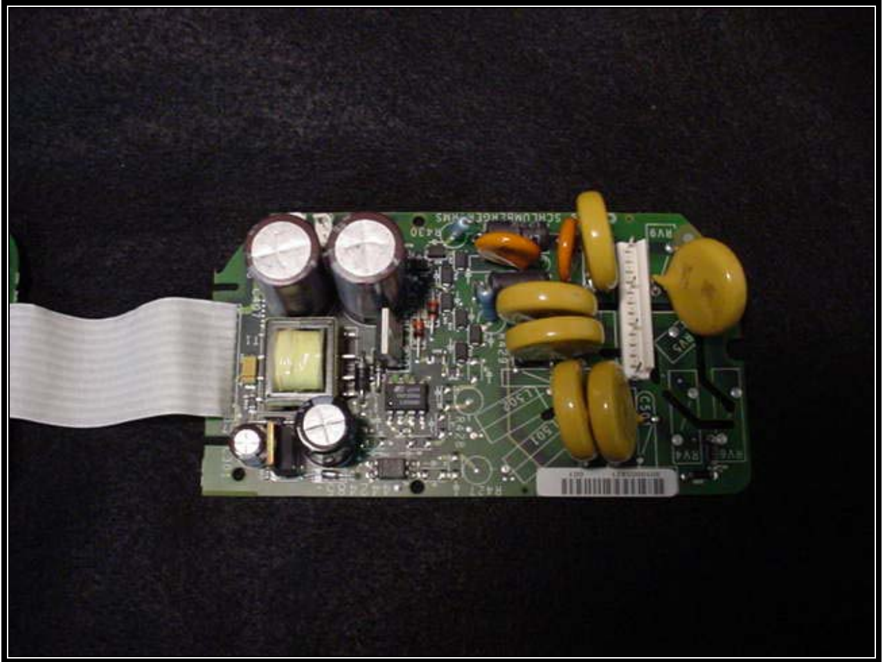
Figure B7: Topside of Power Supply Board
