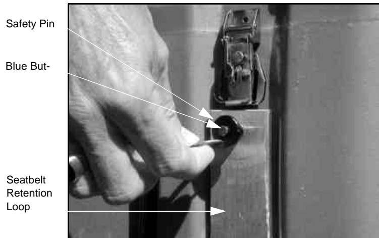
Figure 3.3 Removing the Safety Latch
