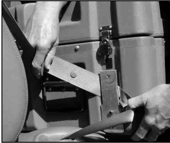
Figure 3.4 Placing Seatbelt in Retention Loop
