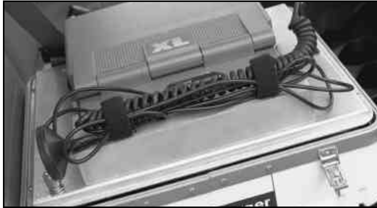
Figure 3.7 Cables retained by Velcro strapping
