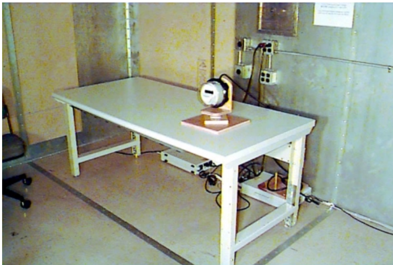
Conducted Emissions Test Setup
