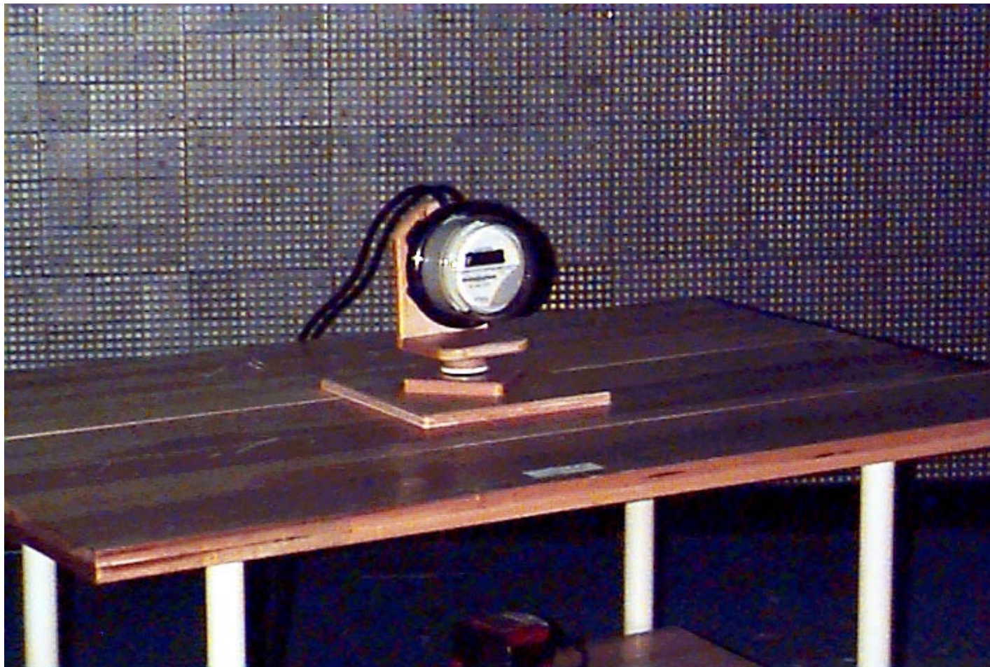
Radiated Emissions Test Setup - Front View
