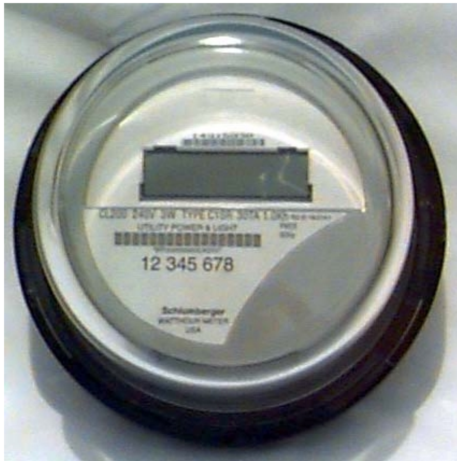
(a) Centron RMR Meter - Back View
