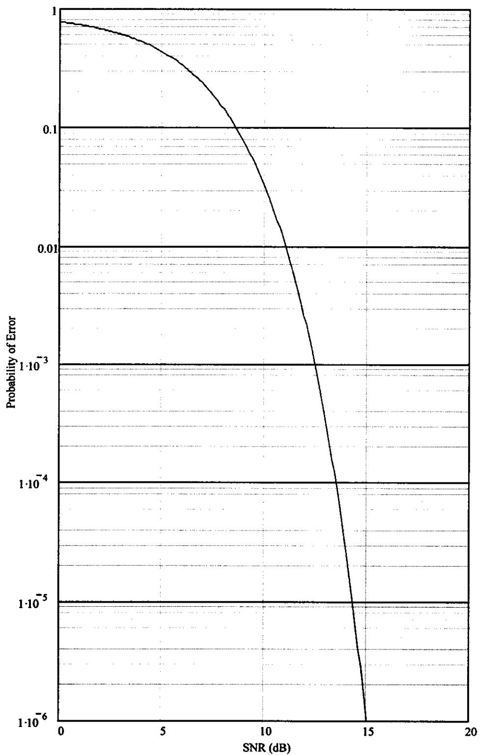
For the threshold error rate of  $2.7 \times 10^{-3}$ , the theoretical Signal to Noise ratio is 11.9 dB.
