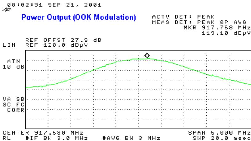
Re-measured power using a direct connection to the EUT: Result = 23dBm
