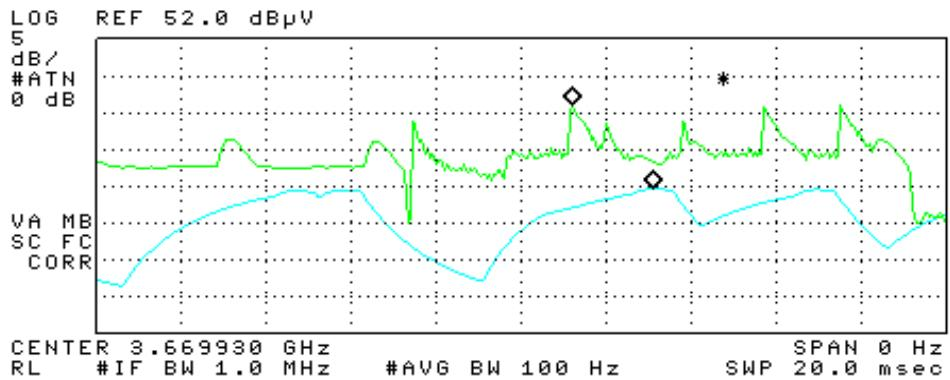
Plots showing peak-to-average differences at the third and fourth harmonics. VBW set to greater than 10Hz as per request of TCB for the "average" measurement.
