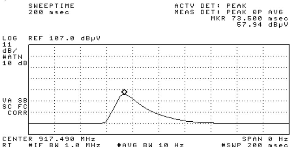
Plots showing peak-to-average differences at the fundamental frequency. VBW set to various values from 1MHz to 10Hz as per request of TCB.
