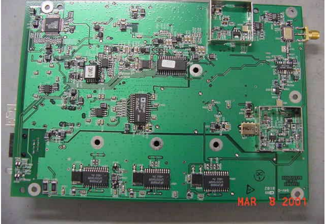
Digital Remote Unit (DRU) Control Board (Bottom) with RF Shields Removed
