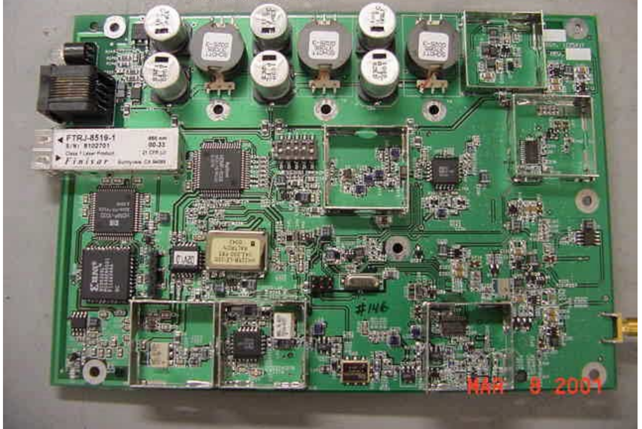
Digital Remote Unit (DRU) Control Board (Top) with RF Shields Removed
