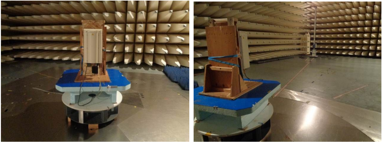
Test setup: Field Strength Emission <1 GHz @10m in the SAC
