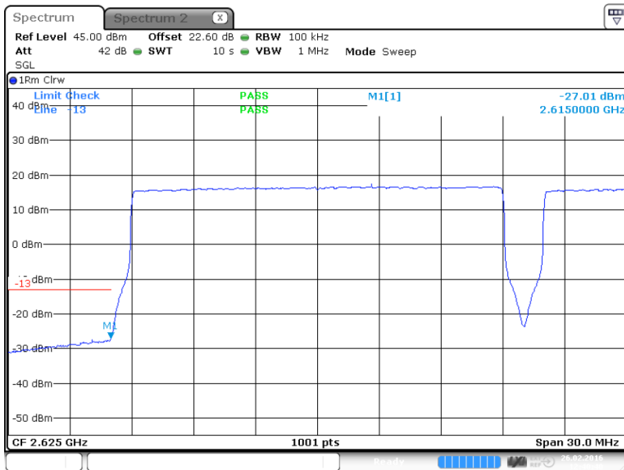
plot 8.3.1.1-#1 Intermodulation: §27.53, §2.1051; Test results; Downlink; LTE Lower Band Edge
